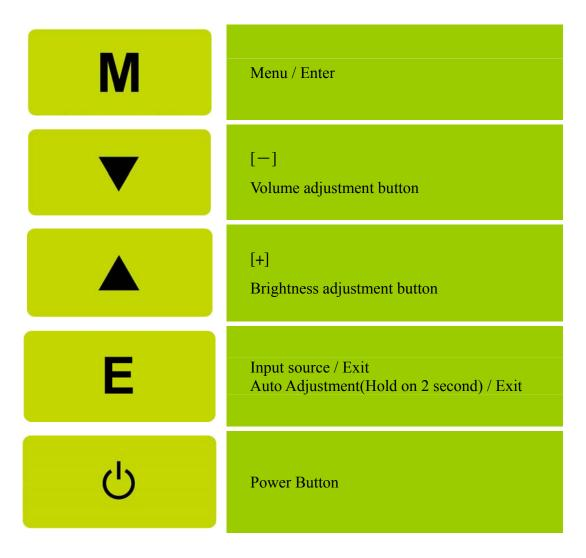
Figure.4. Control Panel Buttons
