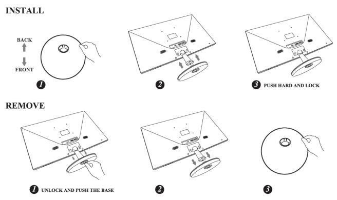
Figure.1. Installing and Removing the Base
