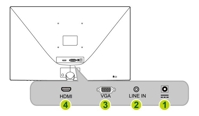
Figure.2. Connecting to a PC
